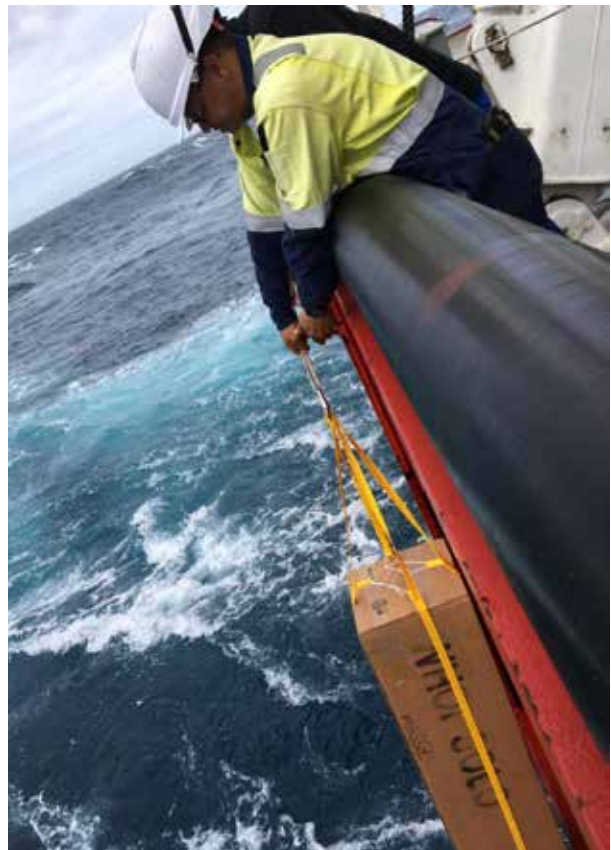
Photo 1: Bosun assisting with the deployment of a SOLO II Argo float from the stern of the SA Agulhas II. Photo credit: Lauren Smith
